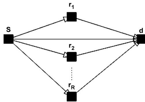
**Fig. 1** Wireless relay network consisting of a source  $s$ , a destination  $d$ , and relays  $R$
