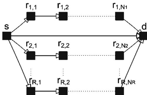
**Fig. 2** Wireless relay network with multihop, multibranch transmission
